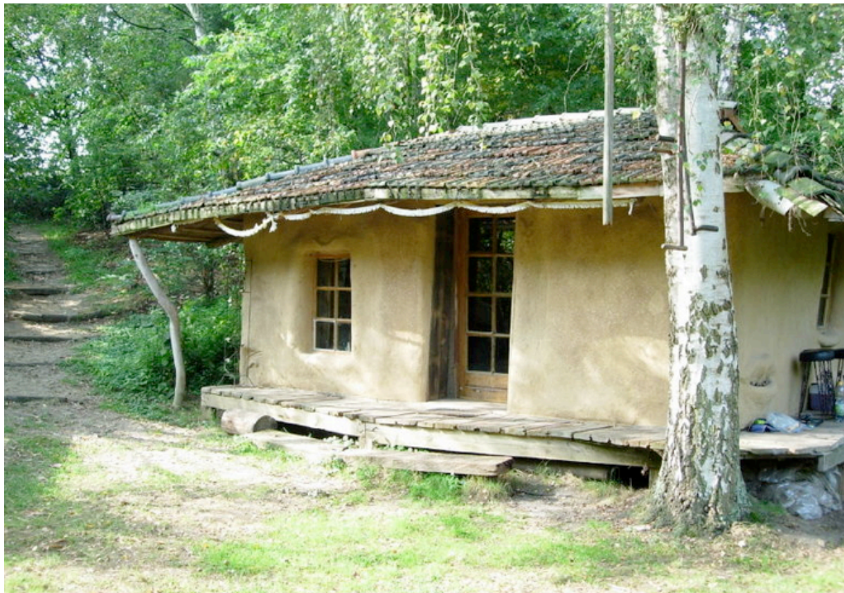
This straw bale house plastered with loam is located in Swalmen , in the southeastern Netherlands
