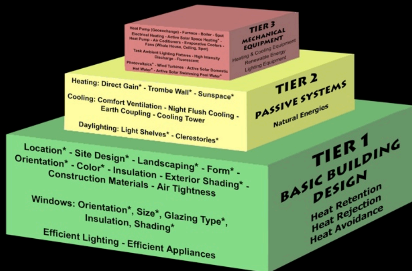
THE 3 TIER APPROACH TO SUSTAINABLE HEATING, COOLING, AND LIGHTING OF BUILDINGS
